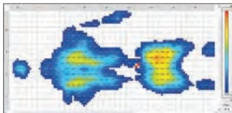
The ergonomic combination of viscoelastic memory foam with multiple-density polyurethane foam was designed and tested with a Pressure Distribution Analyzer, an instrument that measures the pressure at the person-mattress interface. The Pressure Distribution Analyzer is composed of pressure transducers mounted on a flexible base; when set between the person and the mattress, it measures the pressure at the person-mattress interface.
